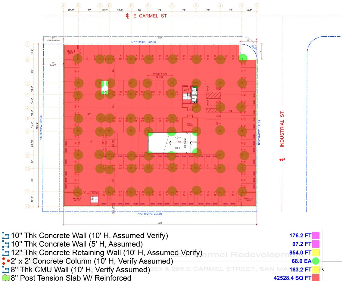
8" Post Tension Slab W/ Reinforced
